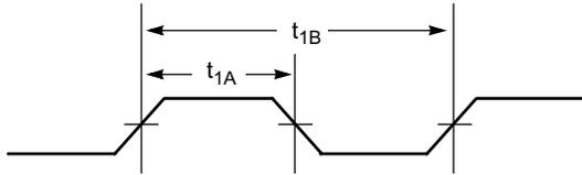
**Duty Cycle Timing (CPU Differential Output)**
