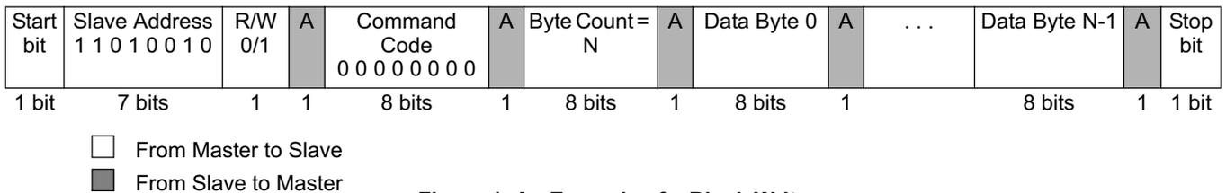
**Figure 1. An Example of a Block Write**
