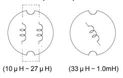
To be connected between #1 and #4, #2 and #3 (10  $\mu$  H ~ 27  $\mu$  H) when using.
