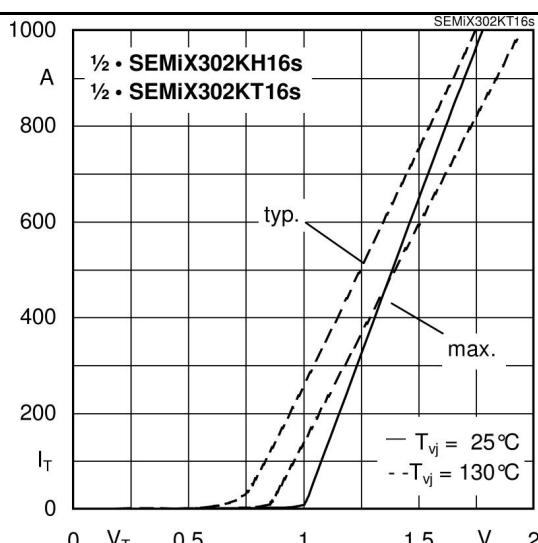
Fig. 7 On-state characteristics
