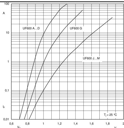
Fig. 1 Forward characteristic ( typical values )
