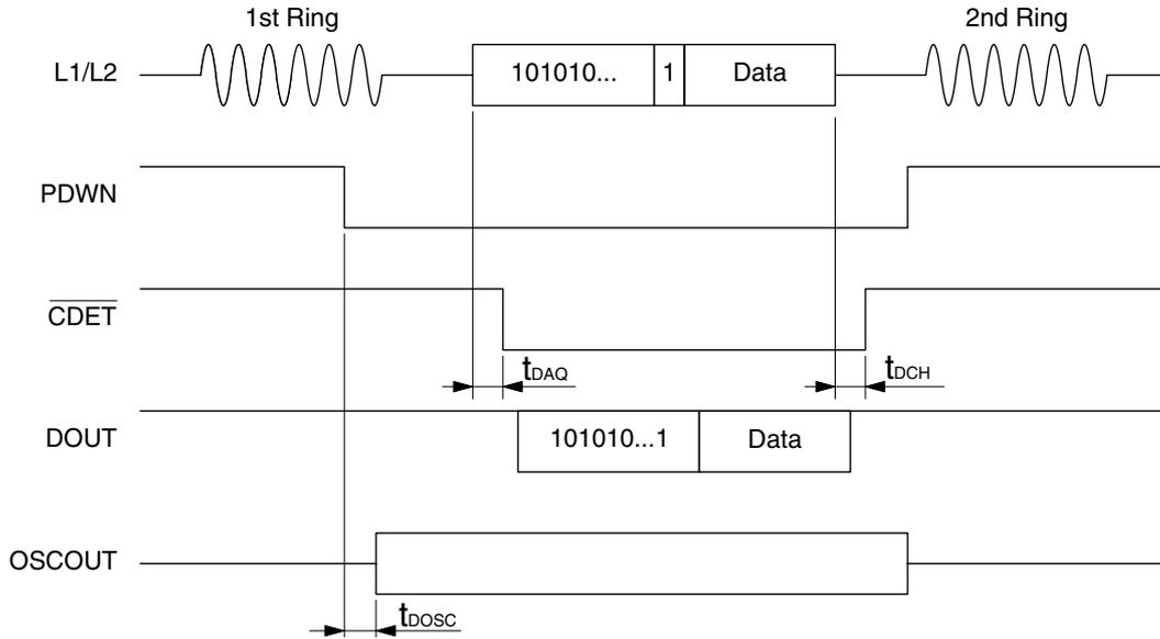
PDWN is an internal signal (set by S0, S1, MODE)
