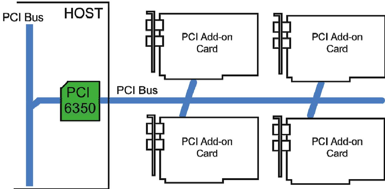
Figure 2. Bus Load Expansion Example
