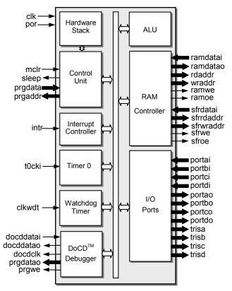
**Timer 0** – Main system's timer and prescaler. This timer operates in two modes: 8-bit timer or 8-bit counter. In the "timer mode", timer registers are incremented every 4 CLK periods. When the prescaler is assigned into the TIMER prescale ration can be divided by 2, 4 .. 256. In the "counter mode" the timer register is incremented every falling or rising edge of TOCKI pin, dependent on TOSE bit in OPTION register.
