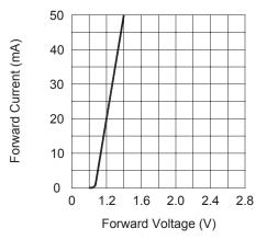
Figure 3. FORWARD CURRENT VS. FORWARD VOLTAGE
