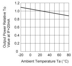
Figure 4. RELATIVE RADIANT INTENSITY VS. AMBIENT TEMPERATURE
