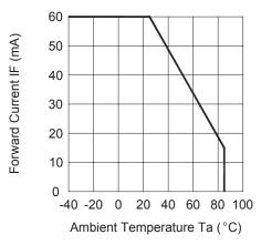
Figure 2. FORWARD CURRENT VS. AMBIENT TEMPERATURE
