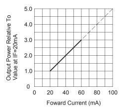
Figure 5. RELATIVE RADIANT INTENSITY VS. FORWARD CURRENT
