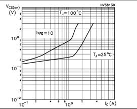
Figure 6. Base-source on voltage
