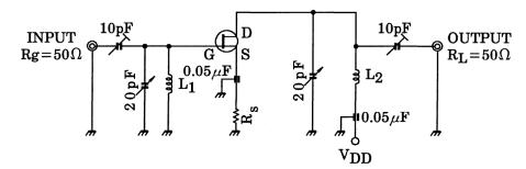
L<sub>1</sub>: 0.8 mm $\phi$  A<sub>g</sub> plated Cu wire, 3 turns, 10 mm ID, 10 mm length.
