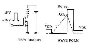
$$\begin{aligned} R_G &= 25~\Omega \\ V_{DD} &= 90~V,~L = 63.4~mH \end{aligned} \quad \quad EAS =$$
