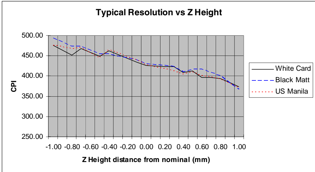
Figure 9. Typical resolution versus height
