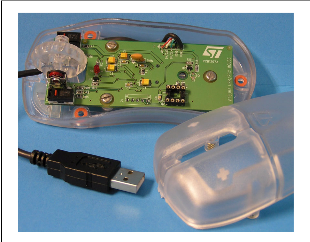
Figure 6. STV-363-R01 - USB/PS2 mouse reference design board
