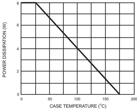
FIG.2- MAXIMUM FORWARD CURRENT DERATING CURVES
