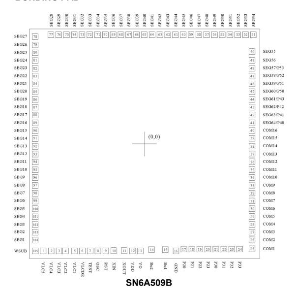
Note: The substrate MUST be connected to Vss in PCB layout.
