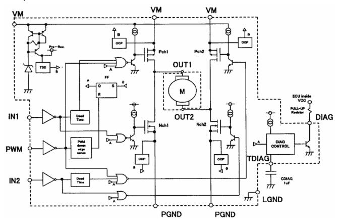
Pre-Reg: Battery inside circuit Dead Time: Protection circuit of length current
