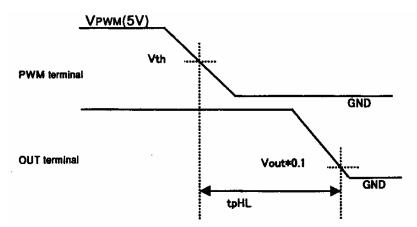
Output transmission time tpLH is time form Vth(2.5Vtyp) of the terminal of PWM to output (Vout\*0.9) Of the output terminal.
