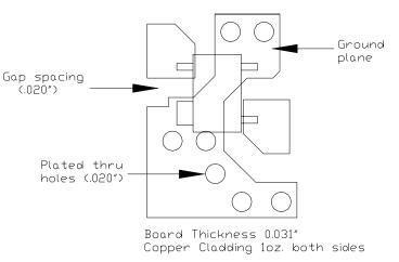
Use multiple plated-through vias holes located close to the package pins to ensure a good RF ground connection to a continuous groundplane on the backside of the board.
