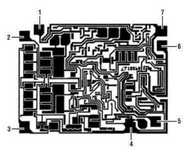
59mils × 78mils, Backlap: 12mils Backside (substrate) is an alloyed gold layer.
