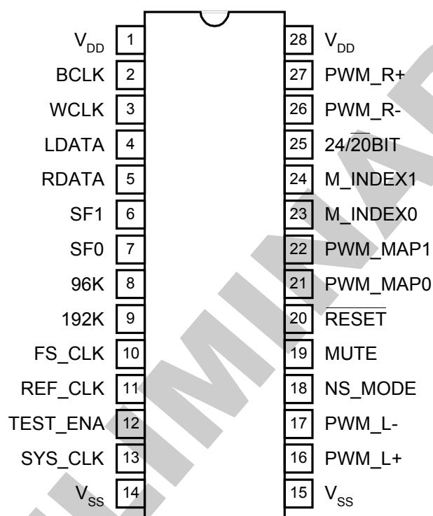
PS9604 (28Lead SOIC, Top View)
