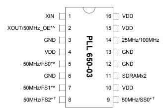
**Note:** SDRAMx2: Double Drive strength. <sup>T</sup>: Tri-Level input ^: Internal pull-up resistor \*: Bi-directional pin (input value is latched upon power-up).
