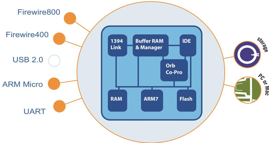
The **Oxford 912** is the latest generation 1394B (Firewire800) to ATA7/ATAPI (IDE) bridge. It supports all PIO, DMA and UDMA modes up to UDMA6, delivering a sustained data transfer performance of over 88MBytes/sec. Hardware features include SBP2.0 acceleration with 'fast start', in addition to dual disk striping and transparent spanning capabilities, all designed to achieve maximum data throughput on Firewire800.
