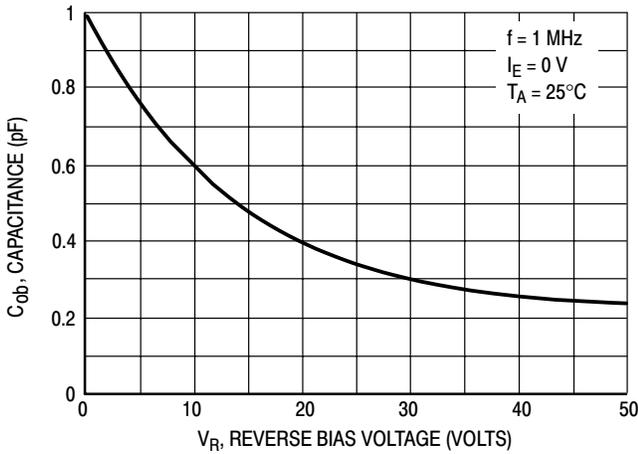
Figure 3. Output Capacitance
