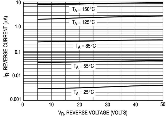
Figure 7. Leakage Current
