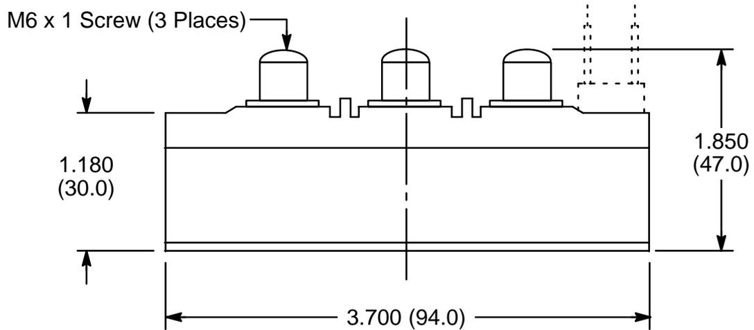
**NOTE:** Can be used with Heat Sink NTE441A
