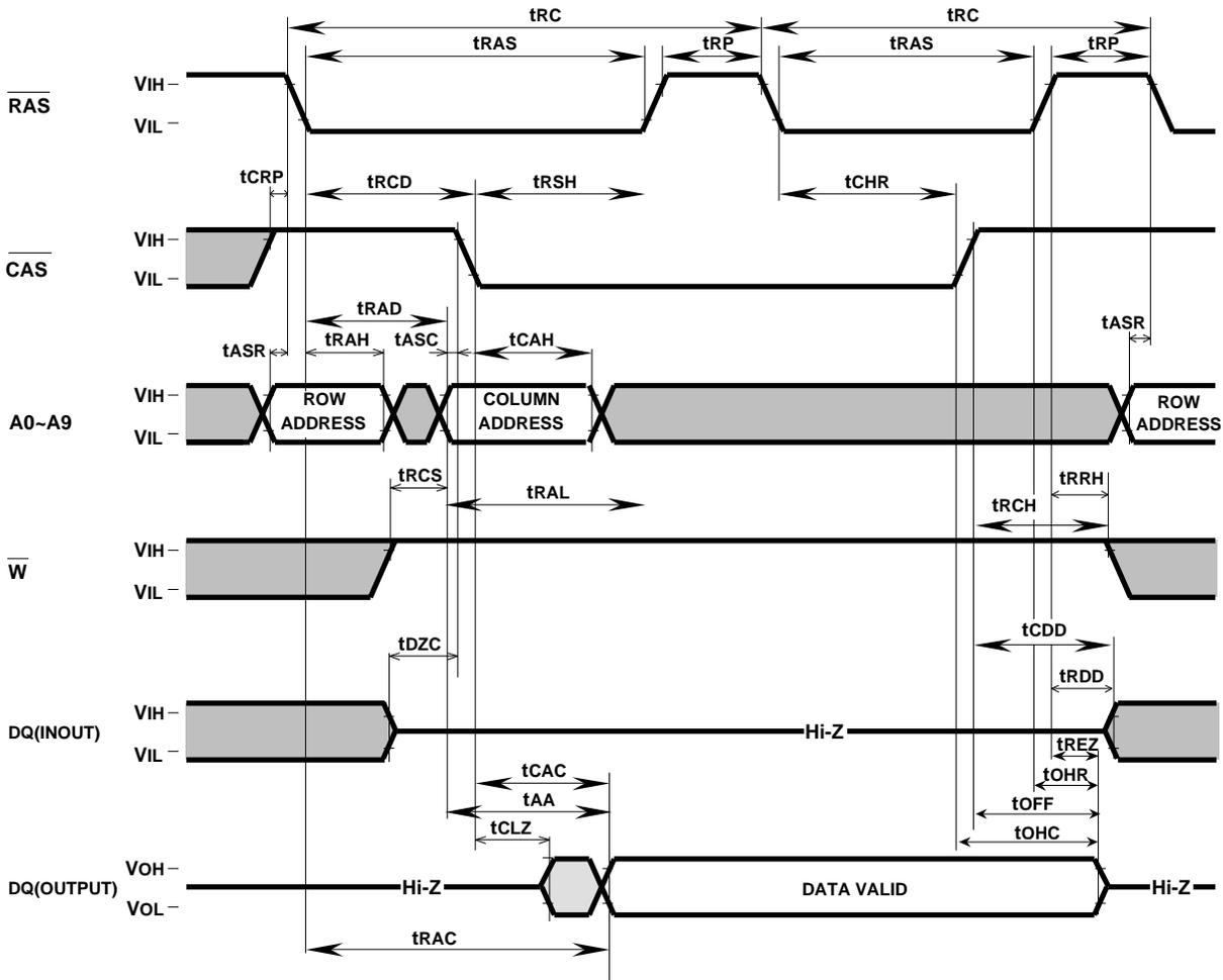
Note 28: Early write, delayed write, read write or read modify write cycle is applicable instead of read cycle. Timing requirements and output state are the same as that of each cycle shown above.
