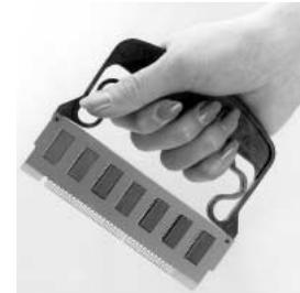
(1) Insert the jig protrusion in the board hole. Grasping the handle, pull the board up.
