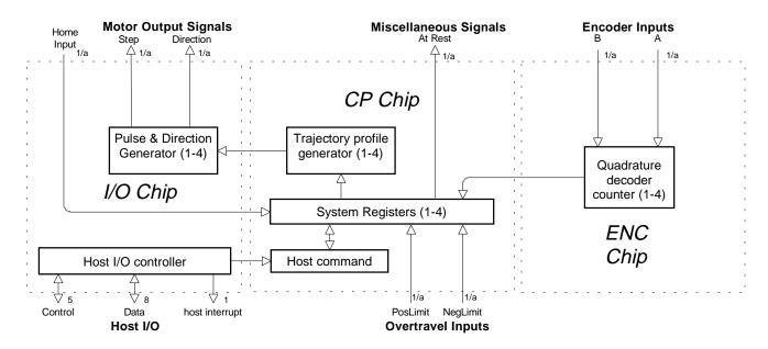
The above figure shows an internal block diagram for the MC1451A and MC1451A-E Motion Processors.
