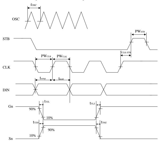
PW <sub>CLK</sub> (Clock Pulse Width)  $\geq$ 400ns t setup (Data Setup Time)  $\geq$  100ns t <sub>CLK-STB</sub> (Clock - Strobe Time)  $\geq$  1 $\mu$ s t <sub>TZL</sub> (Rise Time)  $\leq$  1 $\mu$ s
