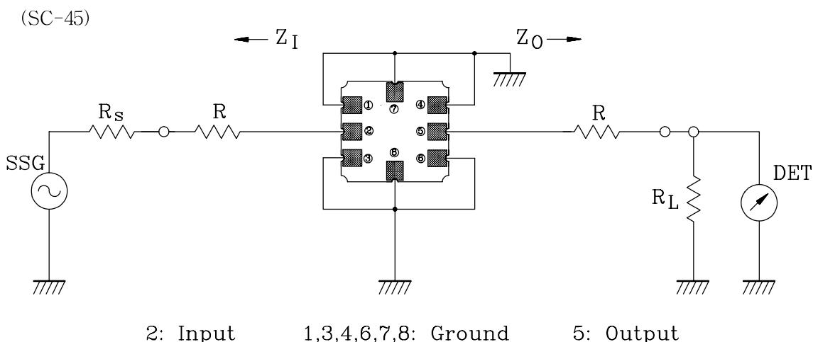
$R_S, R_L : 50\Omega$  (Internal Impedance of Source and Load)
