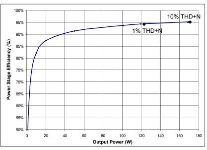
Efficiency vs. output power,  $4\Omega$  single channel driven,  $T_{ambient} = 25 \,^{\circ}C$
