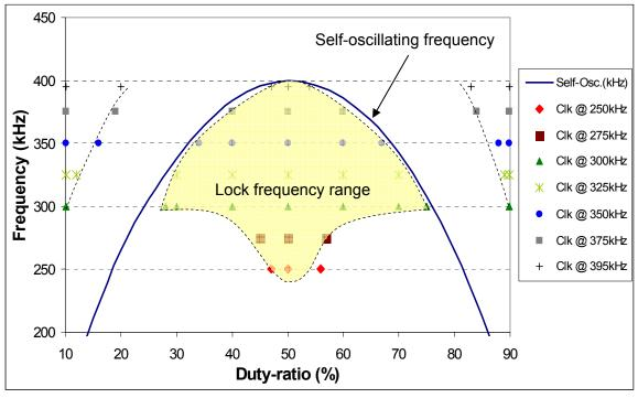
Typical lock frequency range vs. PWM duty ratio for different internal clock frequencies (Self-oscillating frequency set to 400kHz with no input)
