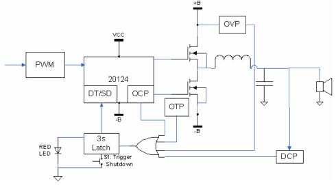
Functional block diagram of protection circuit implementation
