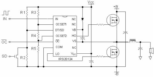
System-level view of gate driver IRS20124S
