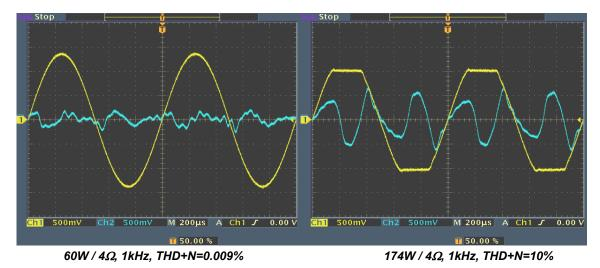
Measured output and distortion waveforms
