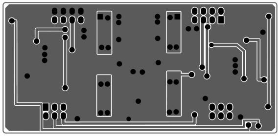
PCB Layout – Bottom layer and pads
