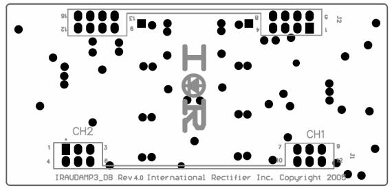
PCB Layout – Bottom-side solder-mask and silkscreen
