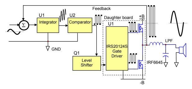
Simplified block diagram of Class D amplifier
