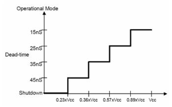
Deadtime / operation mode settings vs V<sub>DT/SD</sub> voltage
