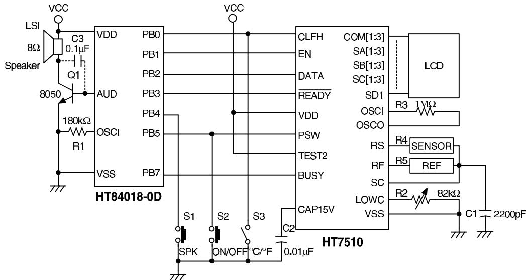
Notes: HT7510's substrate connected to VDD and HT84018-0D's substrate connected to VSS.
