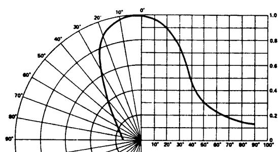
Figure 5. Relative Luminous Intensity
