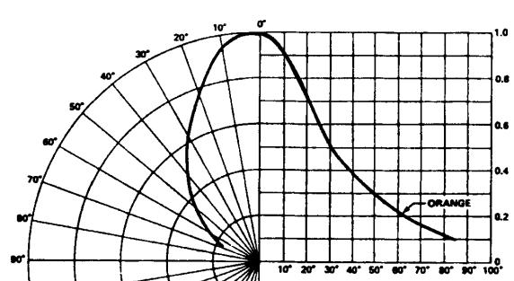
Figure 5. Relative Luminous Intensity
