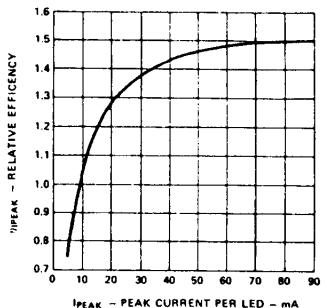
Figure 3. Relative Efficiency
