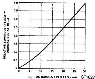
Figure 2. Relative Luminous Intensity
