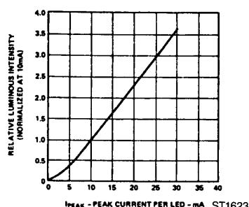
Figure 2. Relative Luminous Intensity vs.
