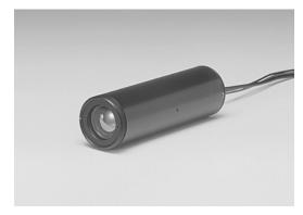
The H7360 series is a wide sensitive area photon counting head device containing a 25-mm (1") head-on photomultiplier tube, high-voltage power supply circuit and photon counting circuit. Since those circuits are designed for wide band, the H7360 series can operate at a high count rate. The high voltage supply for photomultiplier tube and the discriminator level are preset to optimum values so that photon counting can be performed just by connecting a +5 V supply and a pulse counter.
