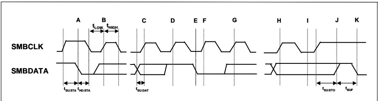
Figure 5. SMBus Read Timing Diagram
