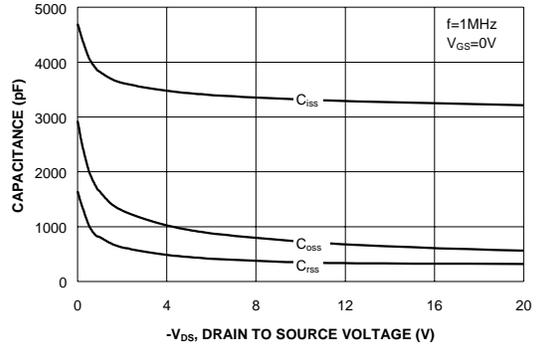
Figure 8. Capacitance Characteristics.
