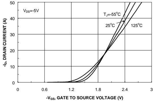
Figure 5. Transfer Characteristics.
