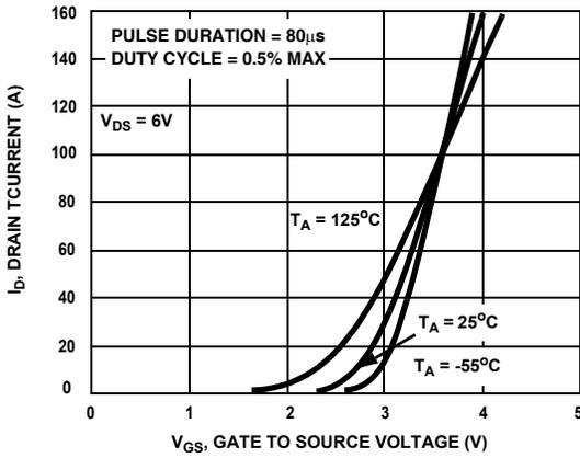
**Figure 7. Transfer Characteristics**
