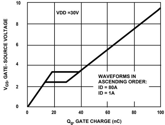
**Figure 14. Gate Charge Waveforms for Constant Gate Current**
