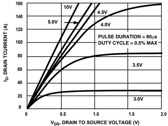
**Figure 8. Saturation Characteristics**
