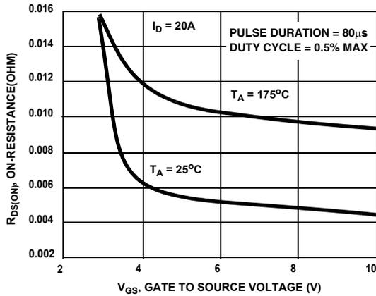
**Figure 9. On-Resistance Variation vs Gate-to-Source Voltage**
