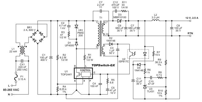
Figure 1. TOPSwitch-GX 12 V, 30 W Universal Power Supply.
