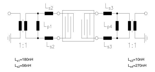
Note: Component values depend on PCB layout.
