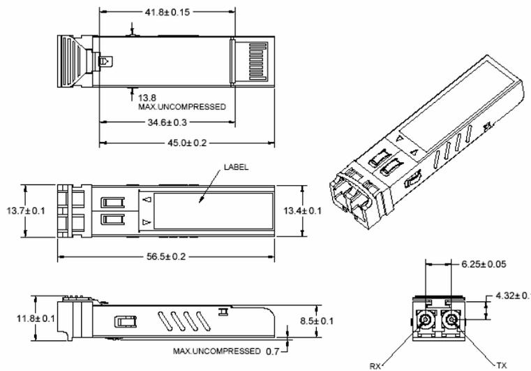
DIMENSIONS ARE IN MILLIMETERS
