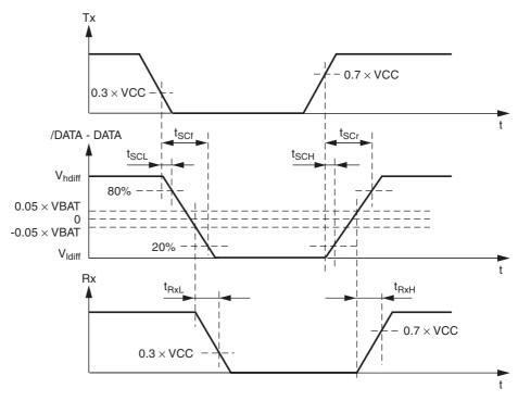
$$\label{eq:Vhdiff} \begin{split} V_{hdiff} &= V_{VBAT} \; (SCI \; driver \; is \; passive, \; recessive \; mode) \\ V_{ldiff} &= V_{T/DATAL} - V_{TDATAH} \; (V_{T/DATAL} \; is \; the \; output \; low \; voltage \; of \; pin \; /DATA) \end{split}$$
