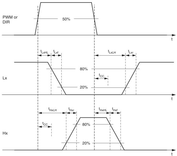
The delays  $t_{\text{HxLH}}$  and  $t_{\text{LxLH}}$  include the cross conduction time  $t_{\text{CC}}.$
