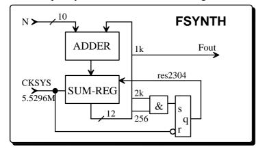
The SC-CLK is defined to be 16 times the center-frequency of the bandpass filters.
