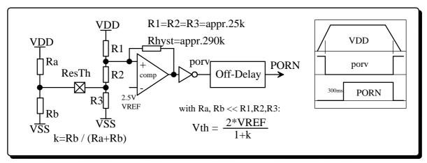
With V(ResTh) defined by external resistors much smaller than R1-3, the POR- threshold can be set in the range of 2.5V to 5.0V according to the given equation.
