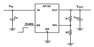
The output voltage is calculated by:
