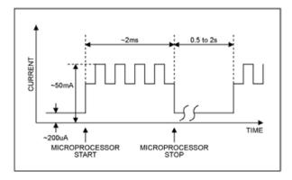
In the standby mode, the microprocessor consumes only around 200 $\mu$ A. Since the phone stays in standby for the longest percentage of time, using a 40 $\mu$ A quiescent current LDO, instead of 140 $\mu$ A, saves 100 $\mu$ A and extends the standby time by 340 $\mu$ A/240 $\mu$ A, or 1.417 times.
