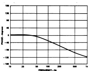
ulator to reject higher order multiples of the reference frequency, the reference frequency of the converter should be at least 2.5 times the closed-loop bandwidth; hence, possible bandwidth is limited by reference frequency used.
