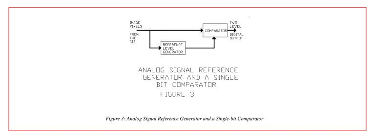
It takes the analog signal from the CIS section of AMIS-710214 and derives a tracking background reference signal. Then this reference is compared against the output signals from the CIS section. The resulting signal from comparison produces a two-level digital signal that is high when the pixel signal is brighter than the background and remains at zero as long as the signal is darker than the background signal.
