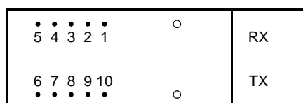
Figure 1. 2417K4A Transceiver, 10-Pin Configuration, Top View
