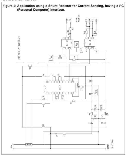
Note: The Serial Interface having a RS232 protocol, has been designed to operate directly with a PC (Personal Computer).
