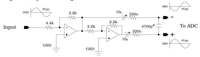
\*Note: Position capacitor as close to pins as possible. Film or high quality ceramic capacitor suggested.
