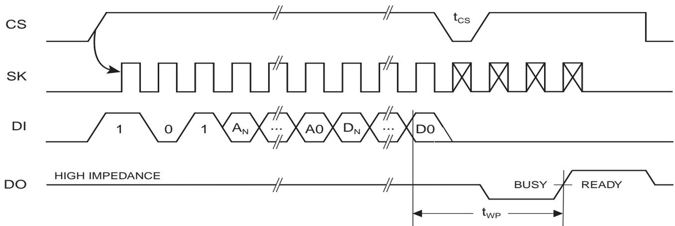
Figure 7. WRAL Timing<sup>(1)</sup>
