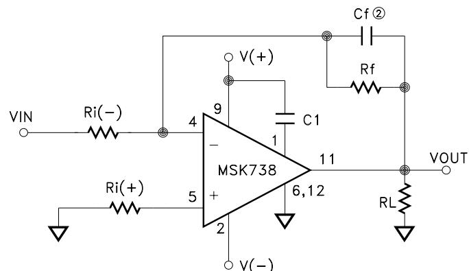
① The positive input resistor is selected to minimize any bias current induced offset voltage.
