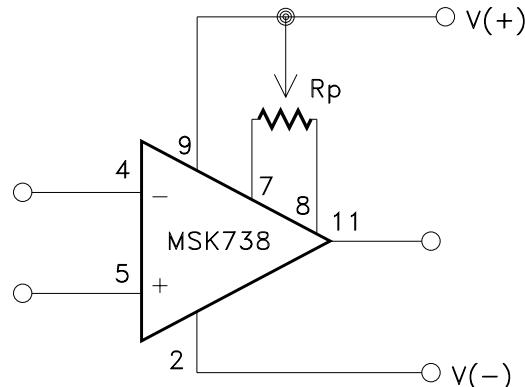
Potentiometer values ranging from 1KΩ to 1MΩ can be used with only a small amount of degradation (typically 0.15 to 0.25µV/°C) of input offset voltage drift. If the input offset voltage is to be trimmed to a value other than "zero", the following formula can be used to approximate the change in input offset voltage drift:
