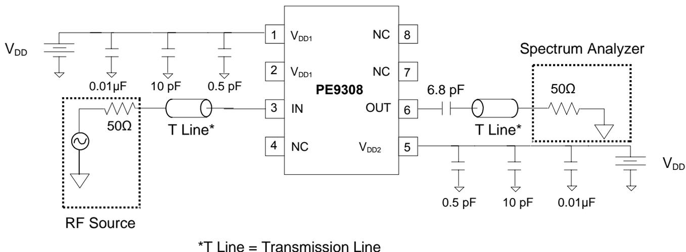
Figure 5. High Frequency System Application
