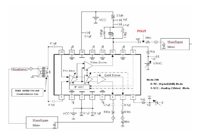
Note Balun Transformer: TOKO 617DB-1714 B4F (Double balanced type)
