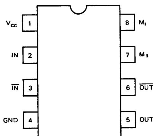
1. V<sub>cc</sub> : Power Supply Pin (+5V)
